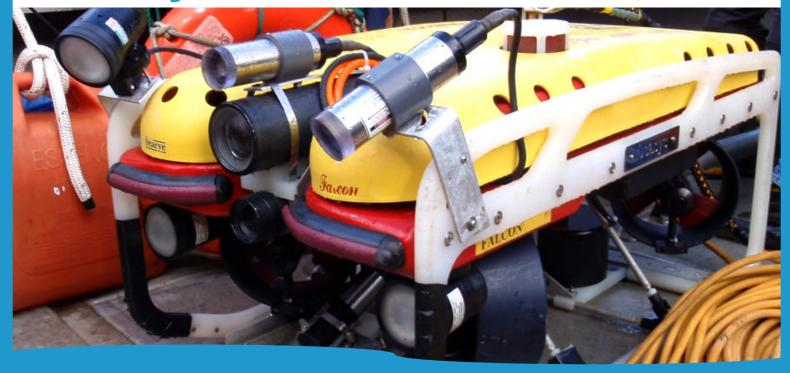
The Seaeye Falcon is the choice of many leading operators for capability, versatility and the ability to get the job done. Lightweight and portable they go where they're needed - inshore, offshore, down tunnels or for flyaway operations. Comes standard with auto-heading & depth.
